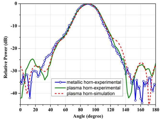
**FIGURE 4** H plane radiation pattern of test horn and corresponding metallic horn [Colour figure can be viewed at [wileyonlinelibrary.com](http://wileyonlinelibrary.com)]
