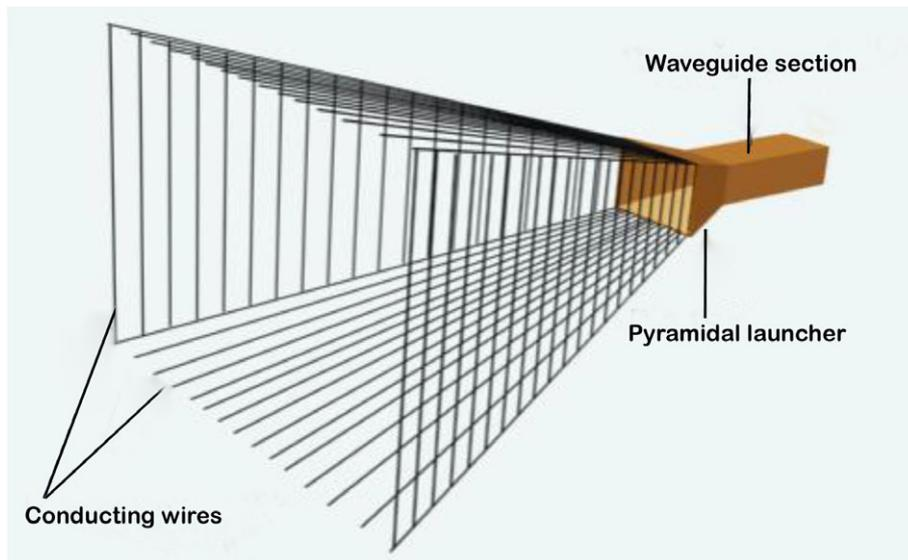
**FIGURE 1** Schematic presentation of proposed plasma horn antenna [Colour figure can be viewed at [wileyonlinelibrary.com](http://wileyonlinelibrary.com)]
