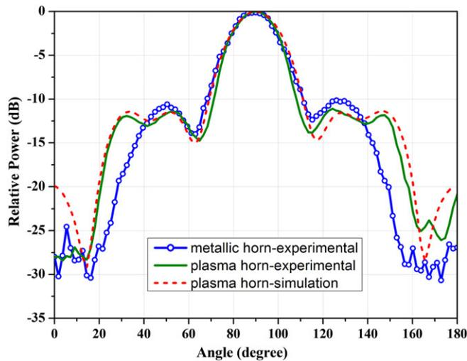
**FIGURE 3** E plane radiation pattern of test horn and corresponding metallic horn [Colour figure can be viewed at [wileyonlinelibrary.com](http://wileyonlinelibrary.com)]
