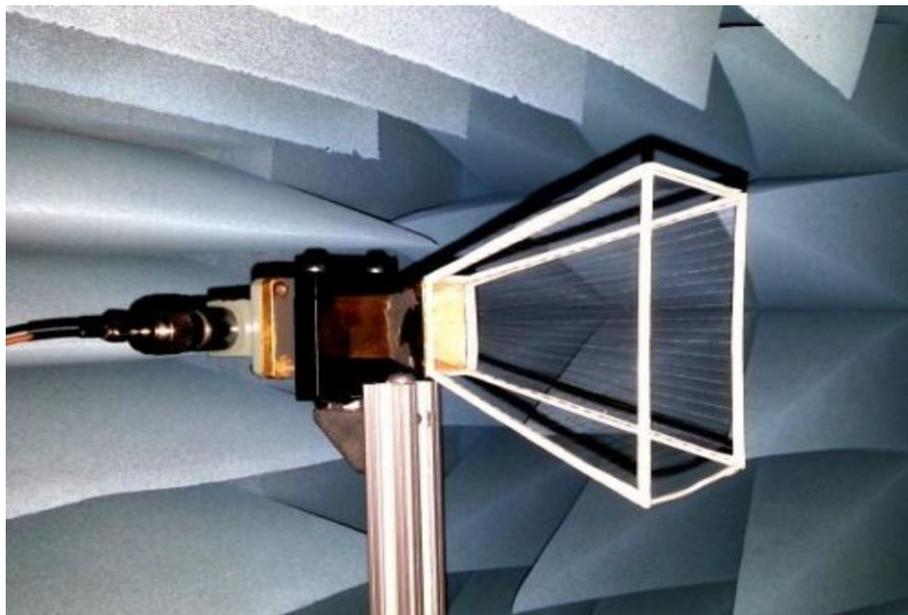
**FIGURE 2** Photograph of plasma horn antenna arranged inside anechoic test box [Colour figure can be viewed at [wileyonlinelibrary.com](http://wileyonlinelibrary.com)]
