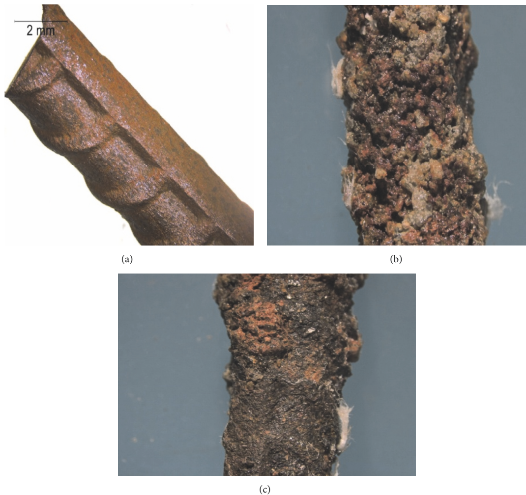
FIGURE 7: Optical micrographs of steel reinforcements: (a) bare, (b) in SAMPLE 1, and (c) in SAMPLE 2.
