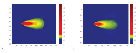
Fig. 2: Radiated electric field distribution near the ENG corner reflector antenna using NS-FDTD for discretization parameter (a) N=8 and (b) N=16
