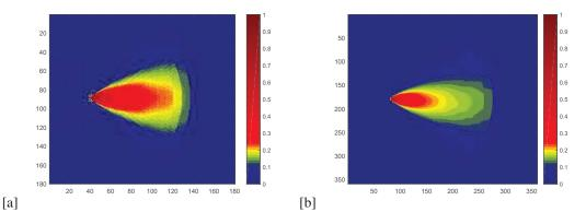
Fig. 3: Radiated electric field distribution near the ENG corner reflector antenna using standard FDTD for discretization parameter (a) N=8 and (b) N=16
