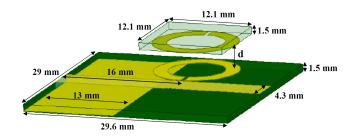
Fig. 1: The layout of BCSRR loaded monopole patch antenna.
