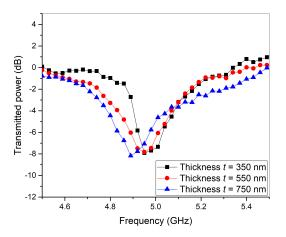
Fig. 2: Magnetic resonance in single square ring SRRs of different thicknesses t of 350 nm, 550 nm and 750 nm respectively made on glass substrate with dimensions - length l=10 mm, width w = 2 mm and split width s = 1 mm.
