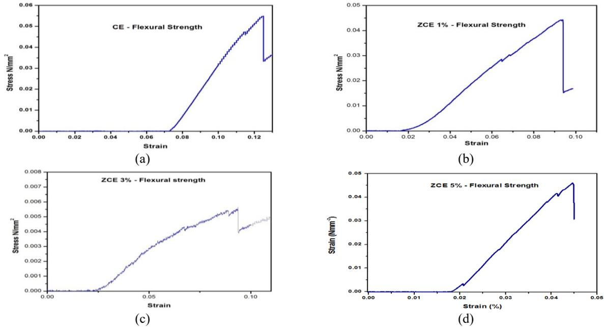
**FIGURE 2.** Flexural strength analysis of the glass fibre reinforced cyanate ester zeolite laminates (a) without zeolite (0 wt %) (b) 1 wt % zeolite (c) 3 wt % zeolite (d) 5 wt % zeolite
