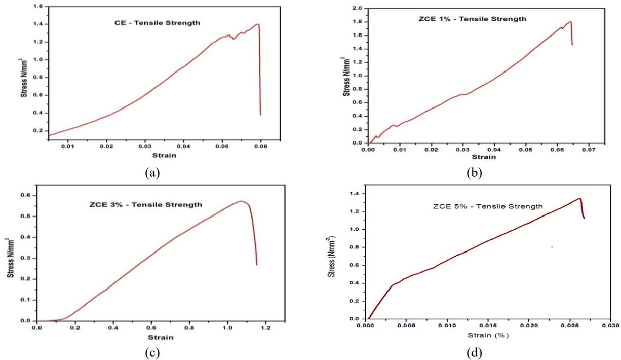
**FIGURE 1.** Tensile strength analysis of the glass fibre reinforced cyanate ester zeolite laminates (a) without zeolite (0 wt %) (b) 1 wt % zeolite (c) 3 wt % zeolite (d) 5 wt % zeolite
