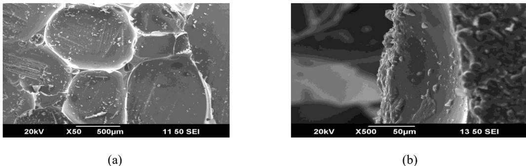
**FIGURE 5.** (a) SEM image of the glass fibre reinforced cyanate ester zeolite laminates with 3 wt % zeolite (b) Cross sectional image
