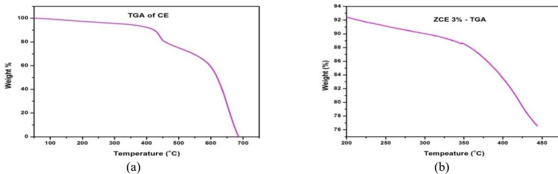
**FIGURE 3.** TGA of the glass fibre reinforced cyanate ester zeolite laminates (a) without zeolite (b) 3 wt % zeolite
