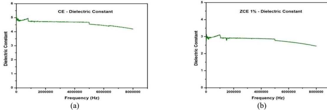
**FIGURE 4.** Dielectric Studies of the glass fibre reinforced cyanate ester zeolite laminates (a) without zeolite (b) 1 wt % zeolite
