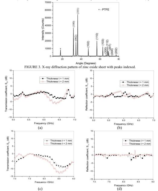
FIGURE 4. Transmission (S<sub>21</sub>) and reflection coefficients (S<sub>11</sub>) of ZnO sheets of different thickness at different frequency ranges[ (a) & (b) in 5 - 7 GHz and (b) & (d) in 7 - 9 GHz ].
