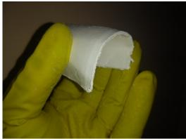
FIGURE 1. Photograph of flexible zinc oxide sheet of thickness 2 mm.
