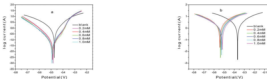
Fig. 8. Tafel plots of MS coupons with and without DmChDa in a) 1M HCl and b) 0.5M H 2 SO 4
