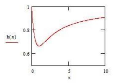
Figure 2. Failure rate function for a=0.001
