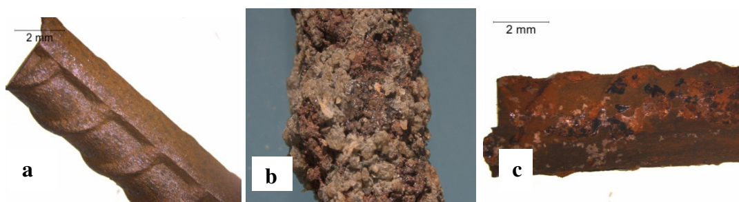
Figure 2.34: Optical micrographs of steel rebars in CPS a) bare b) in the absence of 2APSC c) in the presence of 2APSC
