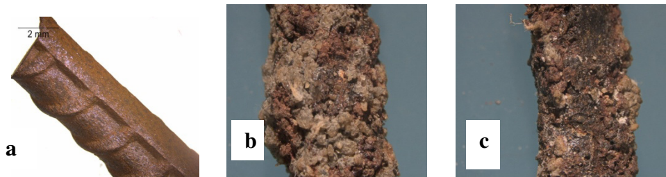
Figure 2.20: Optical micrographs of steel rebars in CPS a) bare b) in the absence of MSP c) in the presence of MSP
