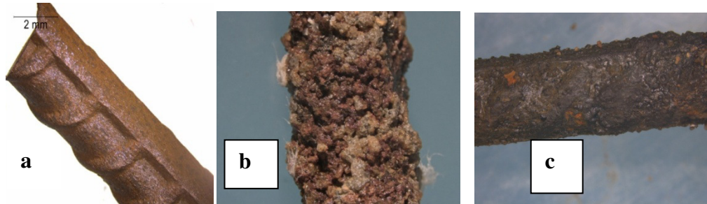
Figure 2.42: Optical micrographs of steel reinforcements a) bare b) in sample 1 c) in sample 4
